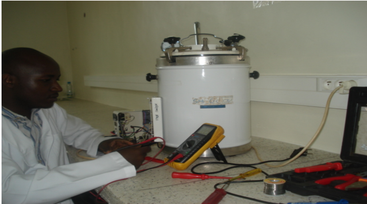
Repair of a small autoclave from microbiology lab
