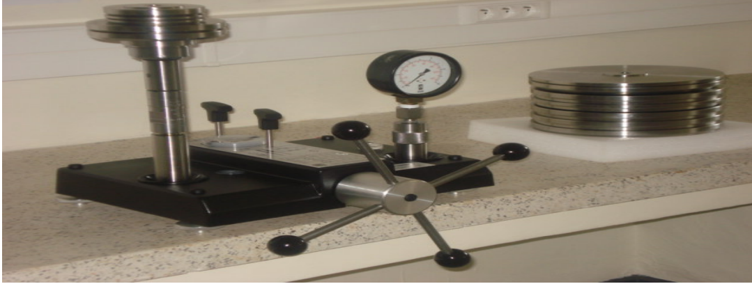
RBS Hydraulic dead weight tester used for calibration of standard pressure gauges
